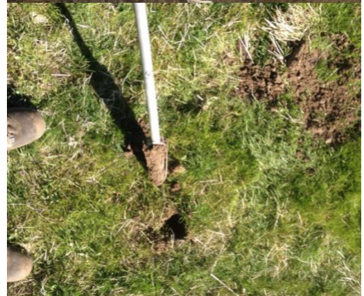
Soil sampling using a spade and hand auger. Soil sampled holes are typically a maximum of 1.2m deep and are backfilled follow the retrieval of a small sample
